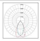
Total Lms: 5425 Lumens Total Input Watts: 65 W Efficacy: 83 Lumens/Watt BUG: B3-U0-G0 CCT/CRI: 4000K/80CRI Maximum Candela: 7024 @ 90°H/10°V
