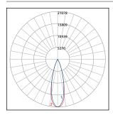
BVG32-L4L60-R22 Total Lms: 5983 Lumens Total Input Watts: 65 W Efficacy: 92 Lumens/Watt BUG: B4-U0-G0 CCT/CRI: 4000K/80CRI Maximum Candela: 21082 @ 92.5°H/1°V
