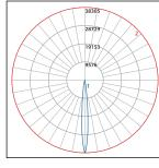
BVS21-L1L15-R9 Total Lms: 1409 Lumens Total Input Watts: 24 W Efficacy: 60 Lumens/Watt BUG: B2-U0-G0 CCT/CRI: 4000K/80CRI Maximum Candela: 38305 @ 0°
