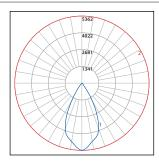
BVS21-L1L35-R55 Total Lms: 3591 Lumens Total Input Watts: 36 W Efficacy: 100 Lumens/Watt BUG: B3-U0-G0 CCT/CRI: 4000K/80CRI Maximum Candela: 5362 @ 0°
