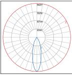
BVS21-L1L35-R30 Total Lms: 3374 Lumens Total Input Watts: 36 W Efficacy: 93 Lumens/Watt BUG: B3-U0-G0 CCT/CRI: 4000K/80CRI Maximum Candela: 9427 @ 0°
